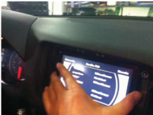
Before fixing the NAViPAD display, line it up.
