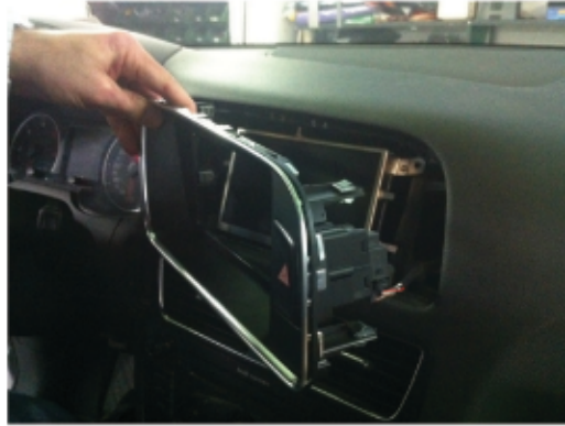
Disconnect the hazard button connector
