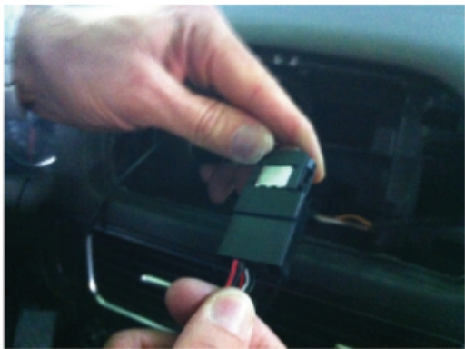
Connect the original display connector to NAViPAD connector
