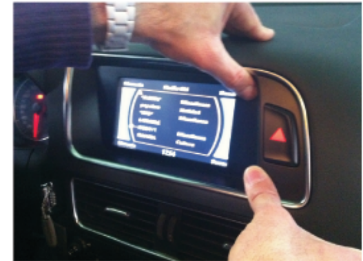
Fix the original display cover protection
