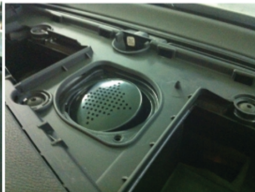
Place the loudspeaker into the central channel housing.
