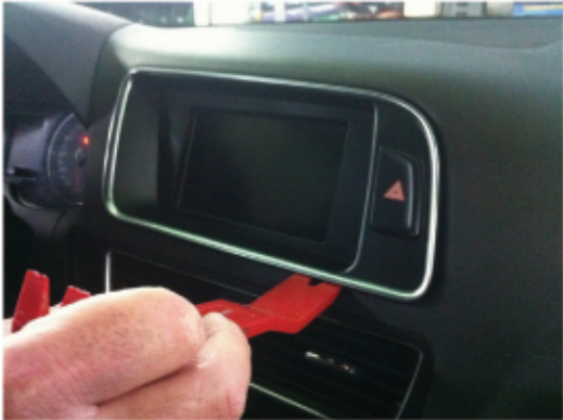
Remove with a plastic lever, the original display cover protection.
