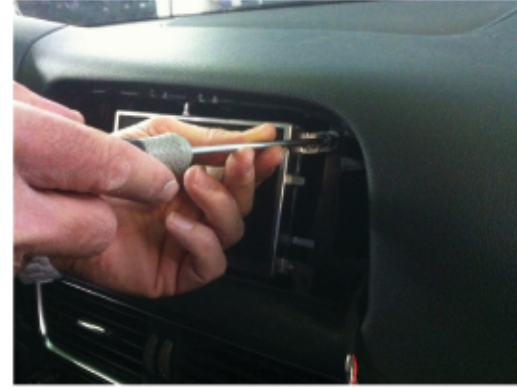
Remove the original display with a Torx screwdriver.
