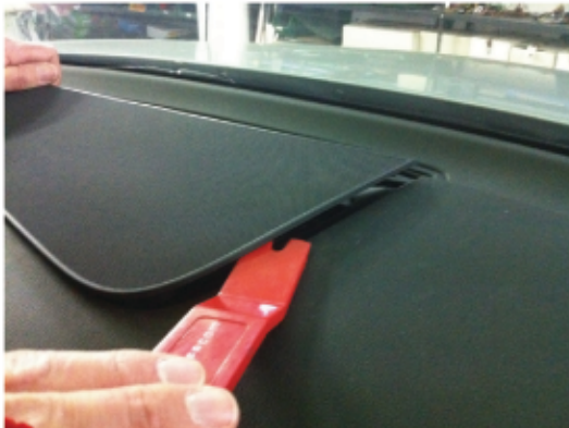
Remove with the same plastic lever, the central channel panel.
