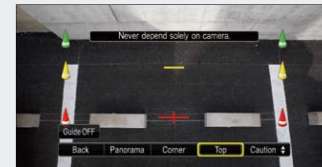
Top view: convenient for precise reversing, for example to hook up a trailer.
